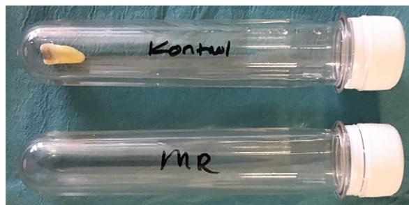
**Figure 2:** Sample tubes containing, top, tooth with dental amalgam in artificial saliva in preparation for testing and, bottom, artificial saliva only. Tube had previously undergone MRI, and the tooth was removed 24 hours after imaging.
