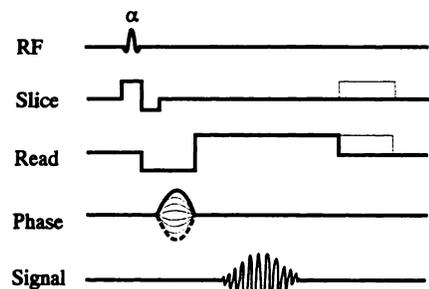
**Figure 2.** The "basic" GRE sequence. See text for details. Dotted gradients along slice-select (section-select) and read provide for resonant-offset averaging.
