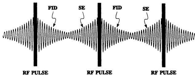
**Figure 1.** A steady-state free precession results when a series of closely spaced RF pulses are applied to a sample. The resultant signal is composed of both FID (free induction decay) and SE (spin echo/stimulated echo) components.
