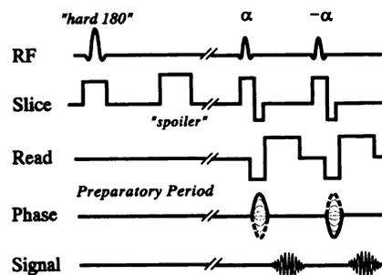
Figure 8. Magnetization prepared GRE sequence (MP-GRE). See text for details.
