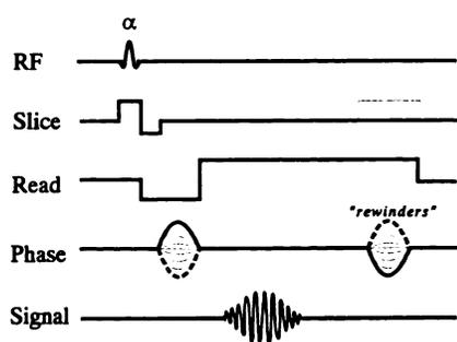
Figure 5. Steady-state GRE sequence with FID sampling (SS-GRE-FID). See text for details.
