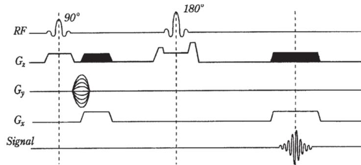
**Figure 1.** Diagram of a conventional spin-echo sequence modified for the MARS technique.  $G_x$  = frequency-encoding gradient,  $G_y$  = phase-encoding gradient,  $G_z$  = section-selection gradient,  $RF$  = radio frequency.
