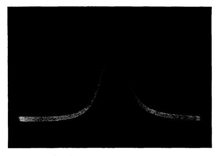
Fig. 3. A resonance line of protons in water, containing MnSO<sub>4</sub> as a paramagnetic catalyst and obtained from the phase component of the nuclear induction signal which corresponds to absorption. The photograph is that of the trace on a cathode-ray oscillograph with the *vertical deflection* arising from the rectified and amplified signal, and the *horizontal deflection* corresponding to different values of the constant field.
